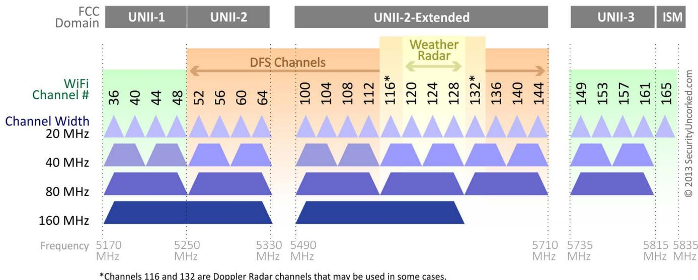
Figure 2. The 5GHz Channel Allocation (image from <http://securityuncorked.com>)
