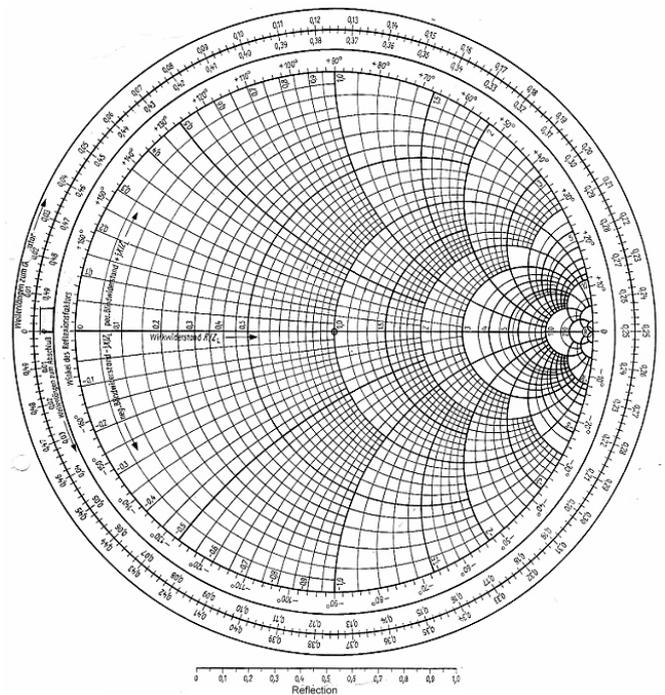
**Figure 1.** With a Smith chart, you can work on problems around transmission lines and circuit matching.
